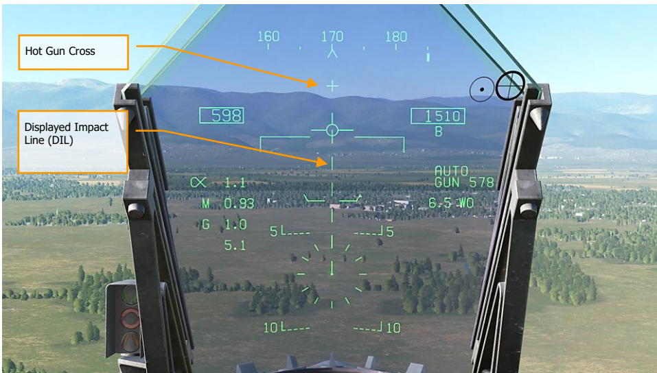
Figure 55. AUTO Bombing HUD, No Designation <7.5 Degree Dive Angle
