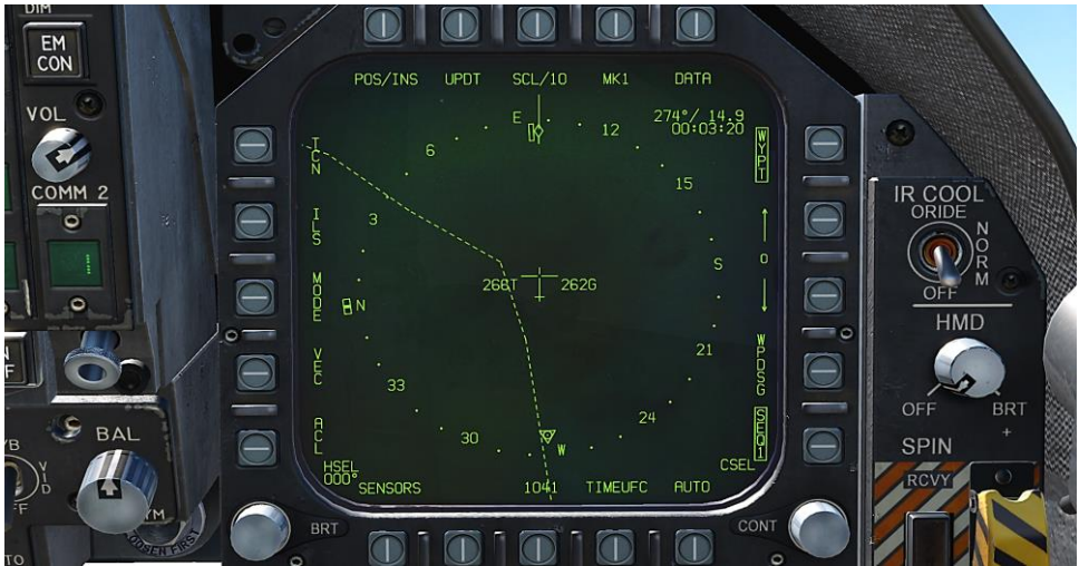
Figure 26. Horizontal Situation Indicator (HSI) Page
