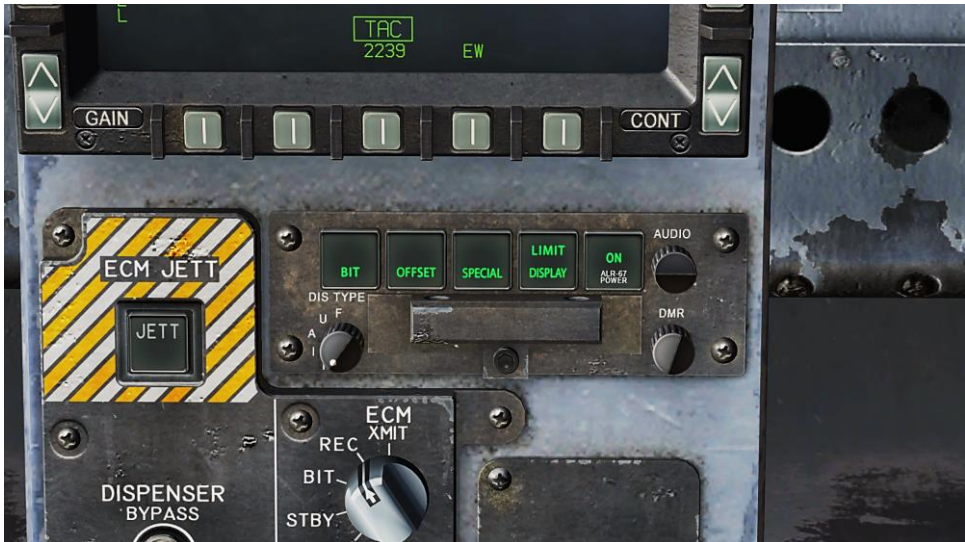
Figure 93. Control Indicator Panel
