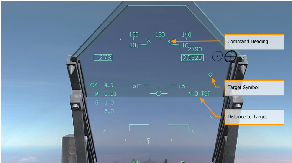
Figure 40. Waypoint as Target on HUD
