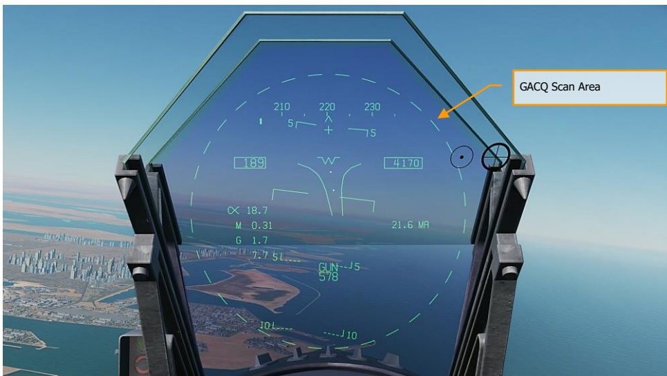
Figure 70. A/A GUNS Auto Acquisition Area
