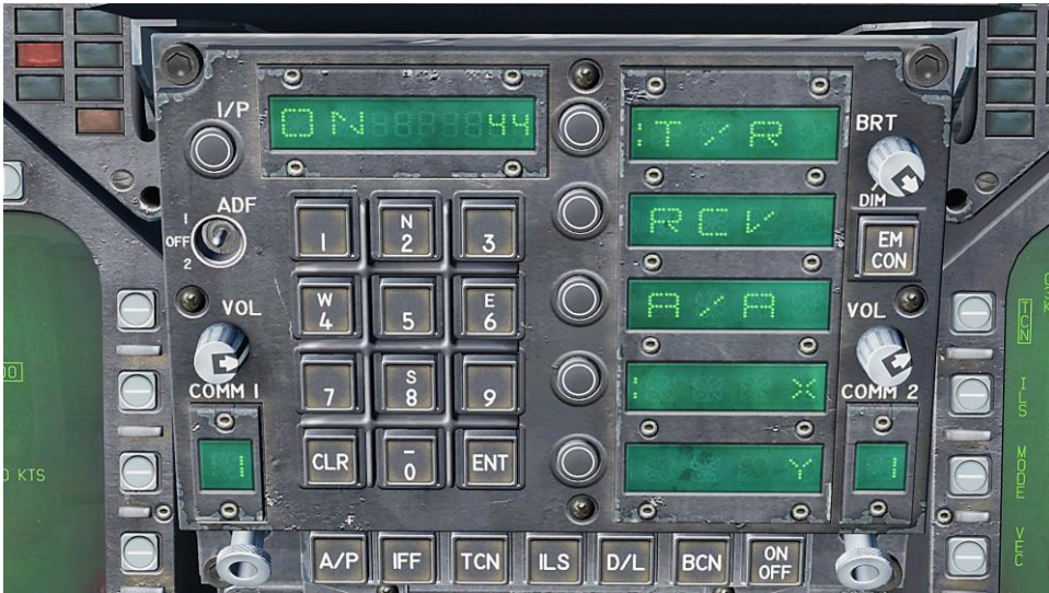
Figure 41. TACAN Options on UFC
