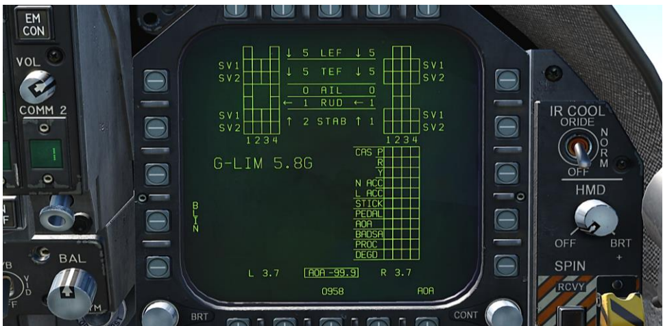
Figure 23. Flight Control System (FCS) Page
