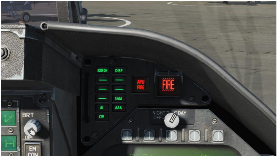
Figure 91. Right Instrument Panel Warning / Advisory / Threat Display Panel
