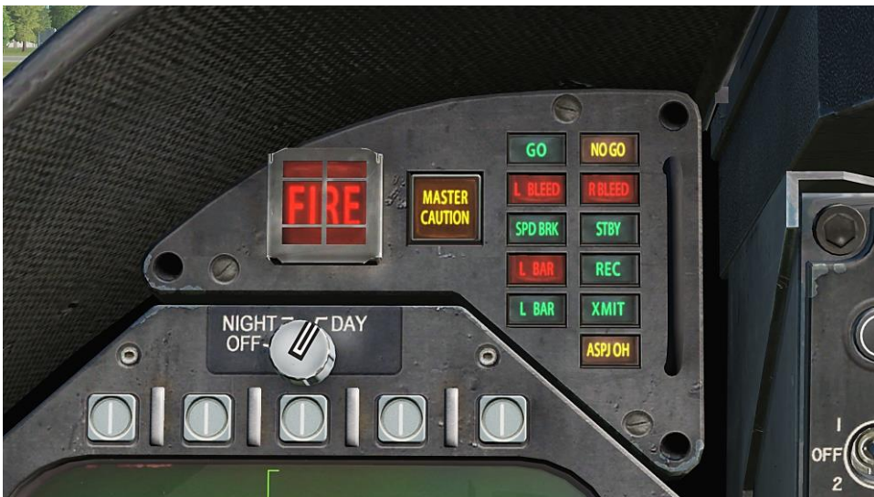
Figure 85. ASPJ annunciator panel
