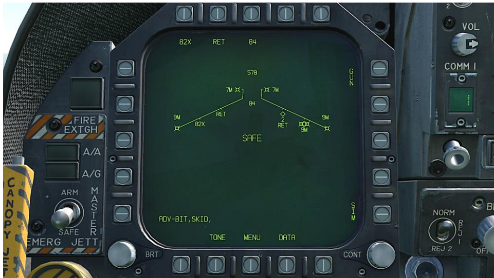
Figure 31. Stores Management System (SMS) Page
