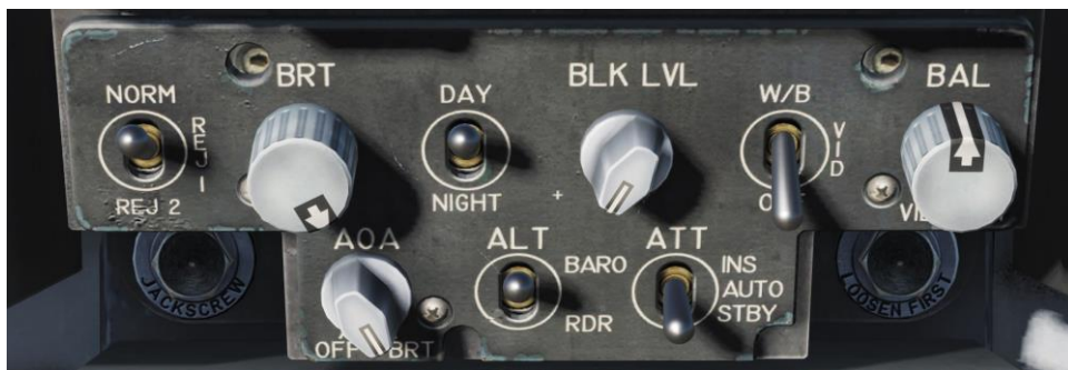
Figure 11. HUD Control Panel
