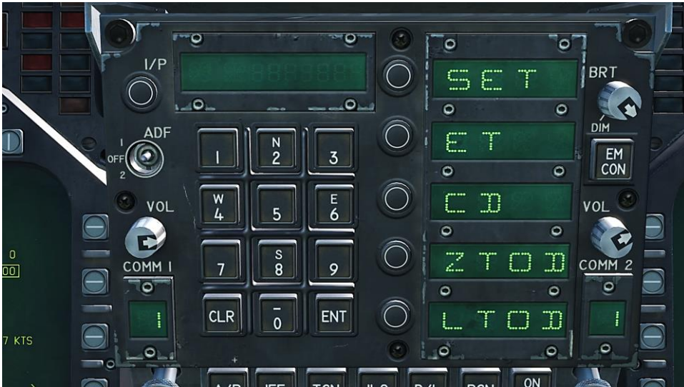
Figure 37. TIMEUFC Options on UFC
