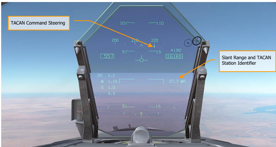
Figure 43. TACAN Steering on HUD
